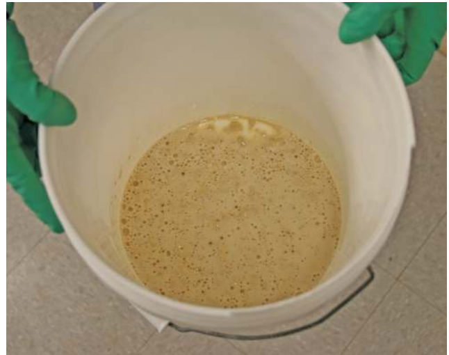
Dissolve EZ-100 powder in a small amount of hot water and bring to volume to make a lukewarm solution.
